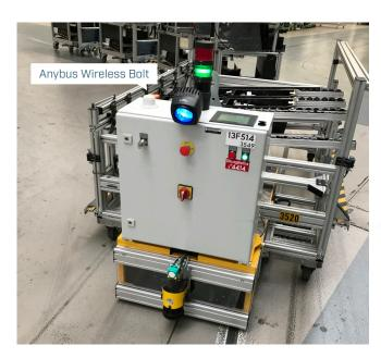
**Safety first.** Not only do the AGVs find their way, they also need to cater for people walking in the corridors and other AGVs in the car factory. Therefore, they are equipped with a laser sensor in the front stopping them if anything comes in the way.
