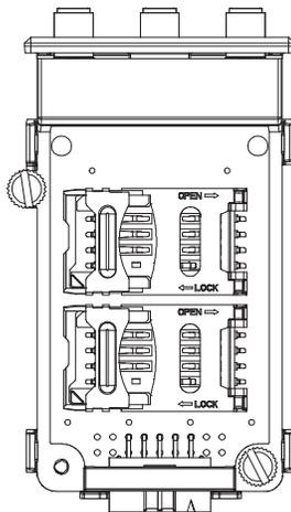
6. Re-install the sled holder containing the sled into the Converter. Make sure it is fully seated.
