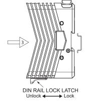
the cradle until flush with the rail and push the DIN rail lock latch to the latched (in) position. For hazardous location installation, the following shall be taken into consideration:
