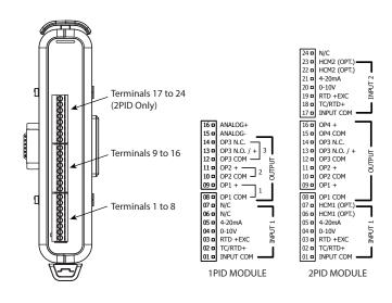
CAUTION: Only UL listed wiring with temperature ratings greater than 90 °C permitted for Class I, Division 2, Zone 2 and ATEX, IECex and UKEX installations.
