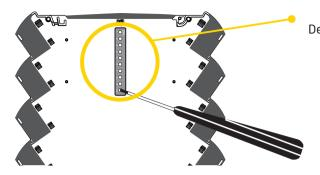
Default factory settings are: Input = 0...20 mA Output = 0...20 mA All DIP-switches in the OFF position
