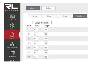
This page allows the user to configure each port with a low and high utilization threshold value in percent. An alarm is triggered when the activity is no longer within the specified threshold range.
