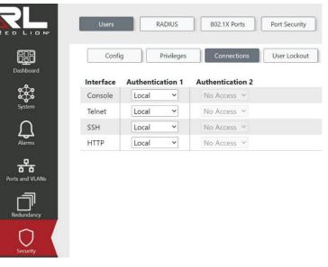
This page allows you to configure how a user is authenticated when they log in to the switch via one of the management client interfaces. The table has one row for each client type.
