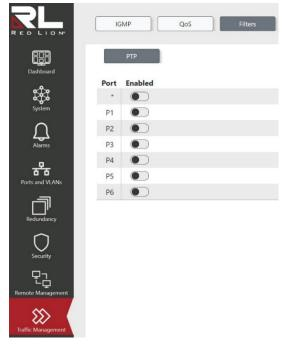
This page allows for the configuration of the PTP traffic filter on a per port basis. PTP frames received on an enabled port will be discarded.
