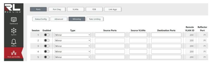
Mirroring is a feature which sends copies of network frames from one port (Rx, Tx, or both) to another port and is often used by administrators in conjunction with a port analyzer to monitor network traffic and analyze or debug network issues.
