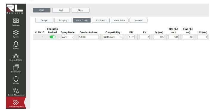
This page allows you to configure IGMP Snooping settings for existing IP Interfaces. New interfaces may be added via the System  $\rightarrow$  IP Interfaces  $\rightarrow$  Interfaces screen.
