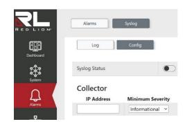
This page allows you to configure the sending of events from the event log, in the form of Syslog messages, to a Syslog collector (also known as a Syslog server).
