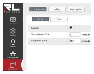
Loop protect, when enabled, detects a loop in the network setup by transmitting Protocol Data Units (PDUs) at a configurable time interval. When received and the PDUs have been determined to be self-generated, then the loop condition can be addressed as configured.
