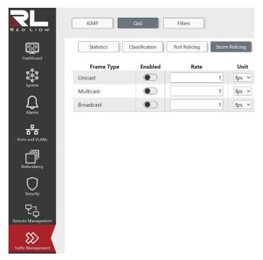
Global storm policing for the switch is configured on this page. There is a unicast storm policer, multicast storm policer, and a broadcast storm policer. These only affect flooded frames, i.e. frames with a (VLAN ID, DMAC) pair not present in the MAC Address table. The settings are defined as follows:
