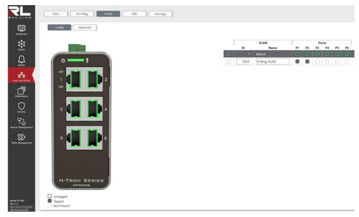
This page allows you to assign ports to VLAN Groups and to configure, for each port/VLAN pair, whether or not frames egressing a port have a VLAN tag.
