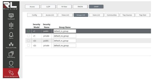
Configure SNMPv3 group table on this page. The entry index keys are **Security Model** and **Security Name**.
