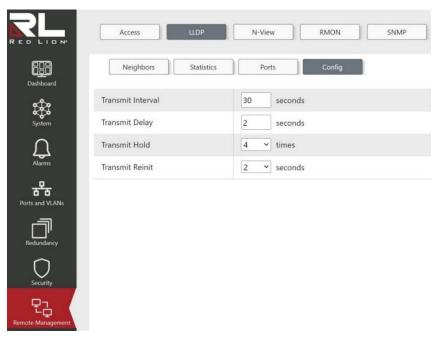
This page allows the user to configure the current LLDP transmit values.
