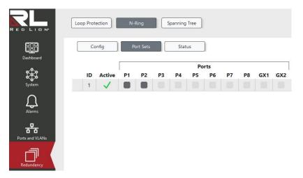
A port set is a group of two ports that may be used for an N-Ring<sup>™</sup>. Click within the table to assign or unassign a port to a port set. The following constraints apply:
