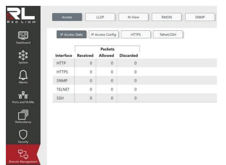
This page provides access statistics for various remote management interfaces. These values are only updated when Access Configuration is enabled via the IP Access Config screen.
