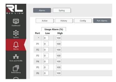
This page allows the user to configure the alarm conditions for each port. The usage ranges below apply to both incoming traffic and outgoing traffic on the port. If either raise above or fall below the set range the alarm will activate.
