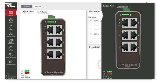
The logical view displays the real status of the system's panel. It can be accessed from the Dashboard and also on any other page by clicking on the left chevron icon at the upper left side of the interface.
