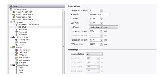
Set the Destination Number to according to the DNP3 network identifier of the target device.
