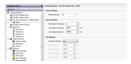
Set the Destination Number according to the DNP3 network identifier of the target device.
