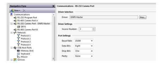
The Source Number setting will serve as an identifier for the Red Lion device on the DNP3 network. Set the Source Number to a number that does not currently exist on the network.
