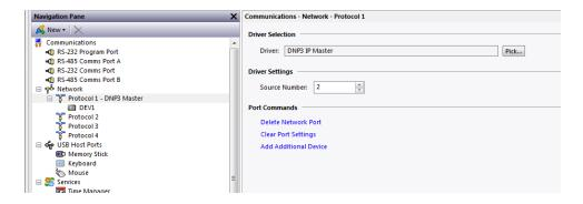
The Source Number setting will serve as an identifier for the Red Lion device on the DNP3 network. Set the Source Number to a number that does not currently exist on the network.
